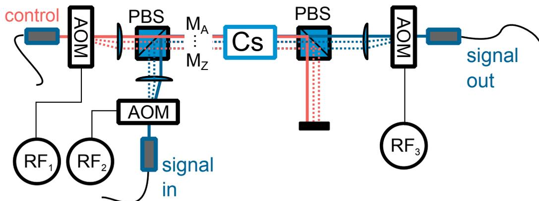
Fig. 1: Sketch of the experimental setup of a multi cell optical memory with storage in different spatial modes  $M_A \dots M_Z$ . AOM: acousto-optic modulator; Cs: Cesium vapor cell; PBS: polarizing beam splitter; RF: radio frequency source.
